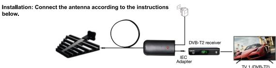
Note: After completing the assembly and installation of the antenna, adjust the antenna to the best position to get a clear TV picture, then secure the antenna and secure the coaxial cable.
