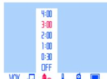
Select any setting through the up and down buttons and confirm with the OK button. Select the setting alarm clock and exit the menu. The alarm clock icon and countdown time icon will be displayed on the right side of the screen. Select off and it will not be displayed.
