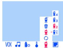
Manual camera selection: enter the manual camera selection submenu, select the added camera by the up and down buttons, and then confirm by the OK button. The screen display interface will switch to the monitoring screen of the selected camera.
