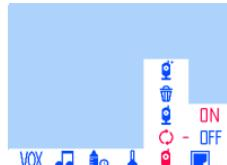
Auto cycle camera display: select the auto cycle setting through the up and down buttons, and then confirm through the OK button. The screen display interface will automatically switch the added camera monitoring screen in sequence.
