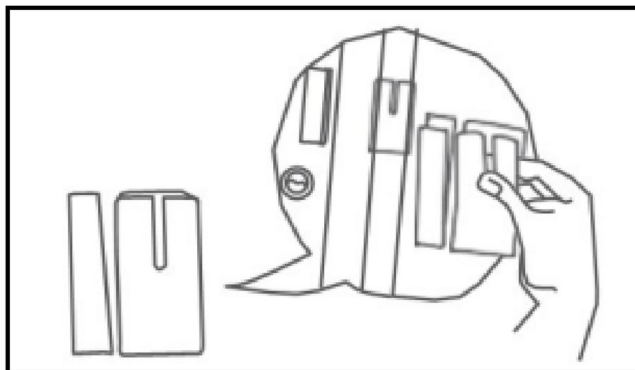
Level installation, installation spacing less than 15 mm.
