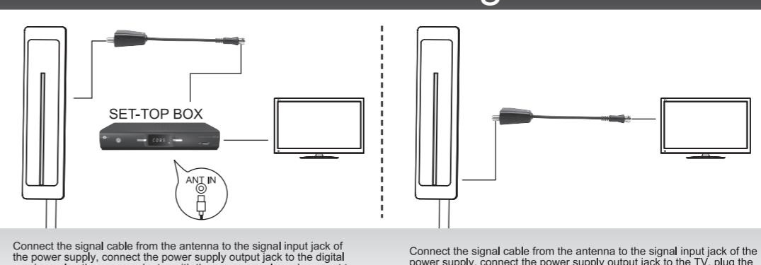
Connect the signal cable from the antenna to the signal input jack of the power supply, connect the power supply output jack to the digital receiver, plug the power adaptor with the power supply and connect to power socket, and finally join the TV and the digital receiver.
