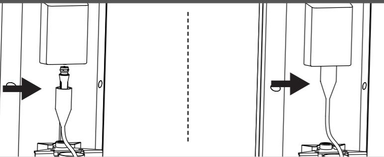
Connect the signal cable to the signal output jack of the antenna and then fix the waterproof cap covering the connections to avoid water filtration.
