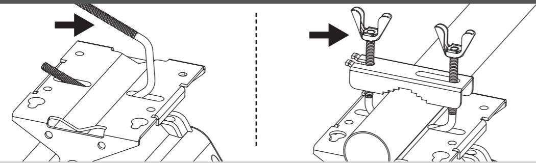
Insert the U-bolt into the hole of antenna bracket and then install the clamp in the U-bolt.
