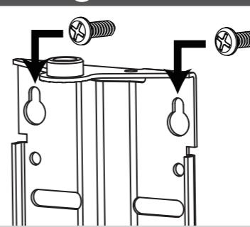
Drill holes and fix screws in the wall according to the holes position on the antenna bracket, attach bracket to the wall and secure with screws.
